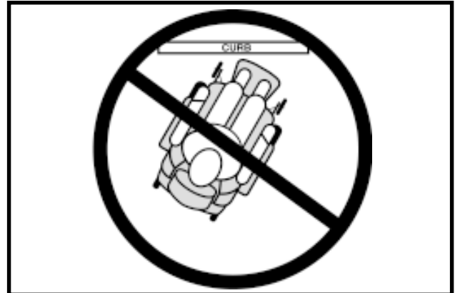
Figure 3. Incorrect Curb Approach
